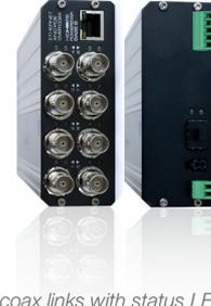
**Front** | 8 coax links with status LEDs, plus a Gigabit uplink port.
