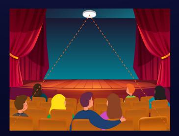
**Detection Radius: 30 meters** Installation height: 3 to 5 meters
