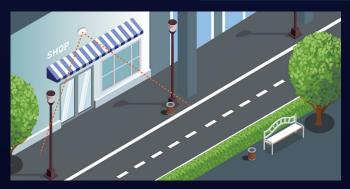
Detection radius: 2 to 15 meters Installation height: 3 meters approximatively
