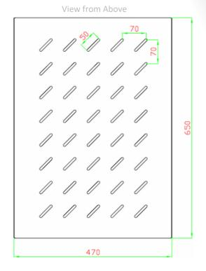
This shelf can be installed in all All-Rack 1000mm deep floor cabinets. It has been specifically designed to fix at the front and rear.
