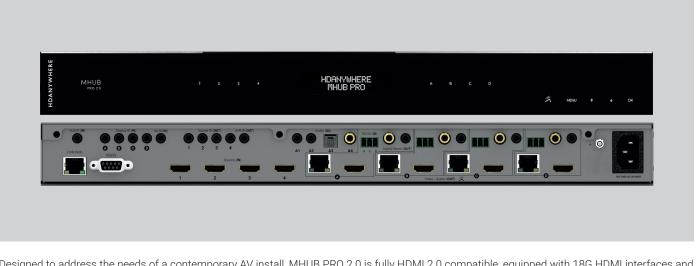
Designed to address the needs of a contemporary AV install, MHUB PRO 2.0 is fully HDMI 2.0 compatible, equipped with 18G HDMI interfaces and backplane to support Ultra HD 4K/60 (4:4:4) with HDBaseT 2.0 technology to transmit 4K to displays up to 40 metres away over a single Cat6 cable with no latency.
