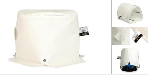
The Lithe Audio Fire hood is designed for use with 6-8'' Round Speakers with a hole Cut-Out Size of up to 210mm. The Fire hood has been designed specifically for in-ceiling speakers and conform with the latest IEE and Building Regulations for Fire integrity of ceilings.
