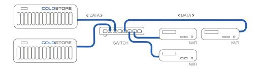
NVRs write to COLDSTORE 3U Pro across the network. Multiple recorders can write to a single COLDSTORE 3U Pro, or one recorder can write to multiple COLDSTORE 3U Pros if required. In principle, individual video streams can be routed to any COLDSTORE 3U Pro on the network as required under the control of the third party recording system.
