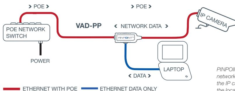
*PINPOINT is inserted between the POE network and the IP camera, diverting the IP camera network connection to the local PINPOINT RJ45 port for a laptop connection.*
