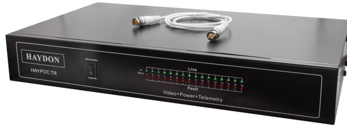
The HAY-POC 16 CHANNEL system provides Power, Video & Telemetry down a single RG59 coax cable. The system is quad based so will carry TVI, CVI, AHD & CVBS (Analogue) up to a 5MP camera signal. The system connects, via provided patch leads, to your DVR. Then simply run your coax cable up to 300 metres and connect to the HAY-POCCAM balun which then provides power 700mA 12Vdc, video & UTC telemetry to your camera.
